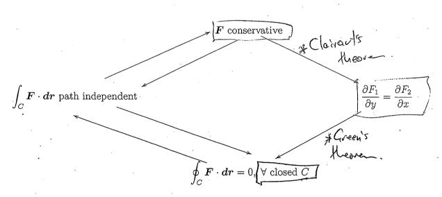
In particular, we now have a test to determine whether or not a given two dimensional vector field is conservative:
