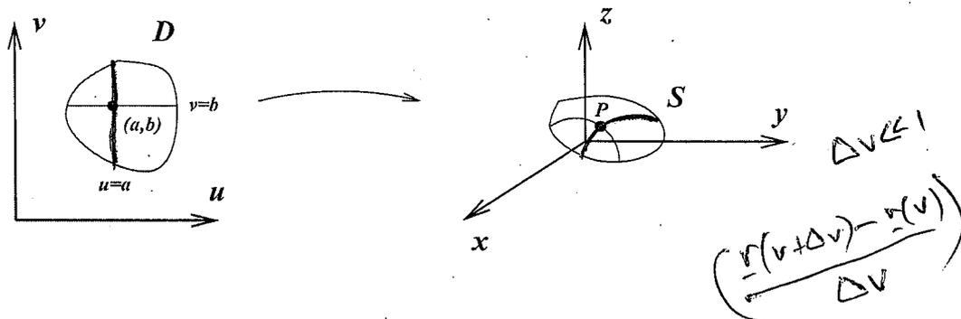
Setting  $u = a$  defines a curve on  $S$  parametrised by  $\mathbf{r}(a, v)$ , for all values of  $v$  such that  $(a, v)$  lies in  $D$ . A tangent vector to this curve at  $P$  is
