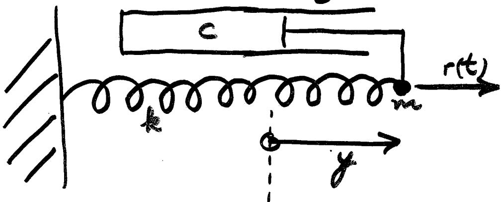
$$m\ddot{y}(t) = \underbrace{-c\dot{y}(t)}_{\text{damping force}} - \underbrace{k y(t)}_{\text{restoring force}} + \underbrace{r(t)}_{\text{applied force}} \quad (23.1)$$
