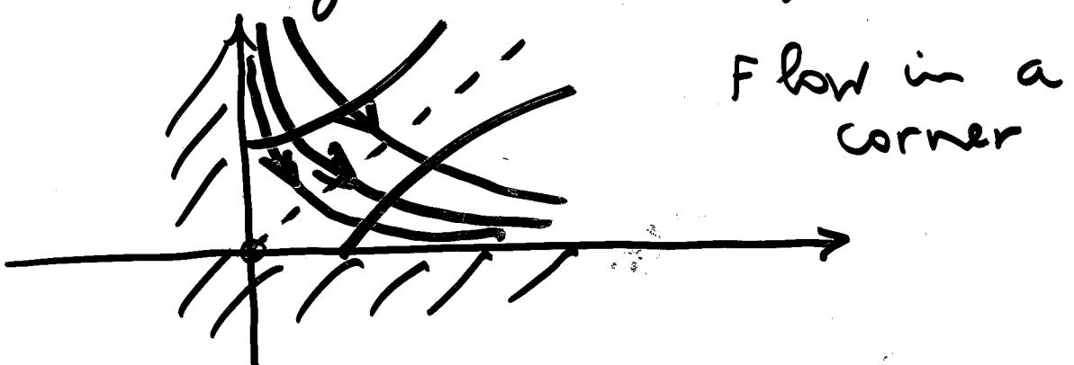
$$\begin{aligned}\varphi(x, y) &= A(x^2 - y^2) \\ \underline{\underline{v}} = \underline{\underline{\nabla}}\varphi &= 2Ax\hat{i} - 2Ay\hat{j}\end{aligned}\quad \left. \begin{array}{l} x > 0 \\ y > 0 \end{array} \right\}$$
