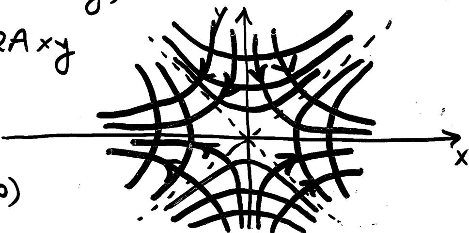
An unlikely looking flow pattern. But note can put an impenetrable wall along any streamline without changing pattern. So we get solution for:
